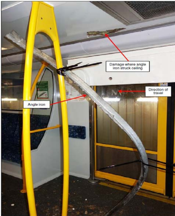
Figure 3: Angle Iron secured inside carriage N5222
