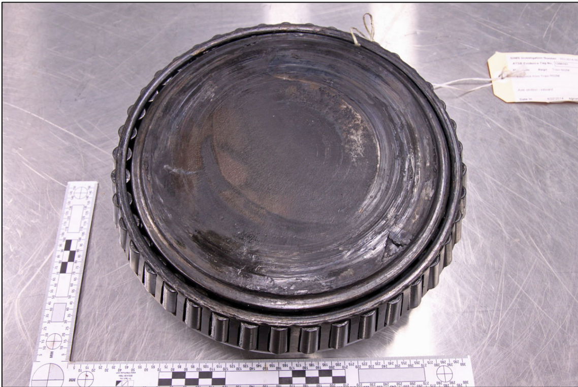
Figure 6: View of the fractured axle adjacent the low speed bearing
