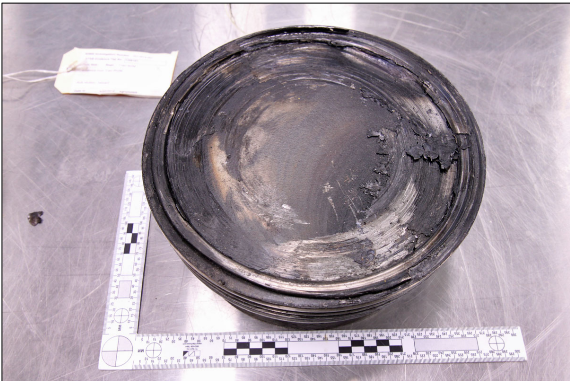
Figure 5: View of the fractured axle adjacent the oil flinger
