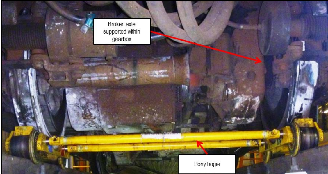
Figure 5: Axle supported by pony bogie after recovery
