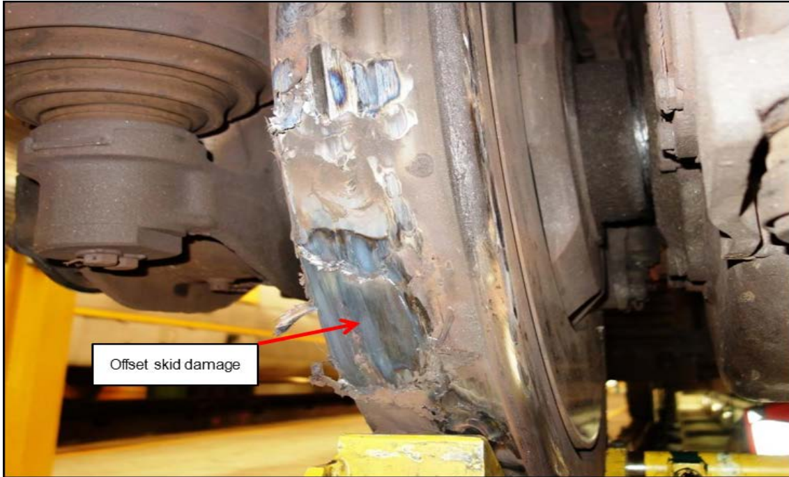
Figure 11: Damage to No. 8 wheel
