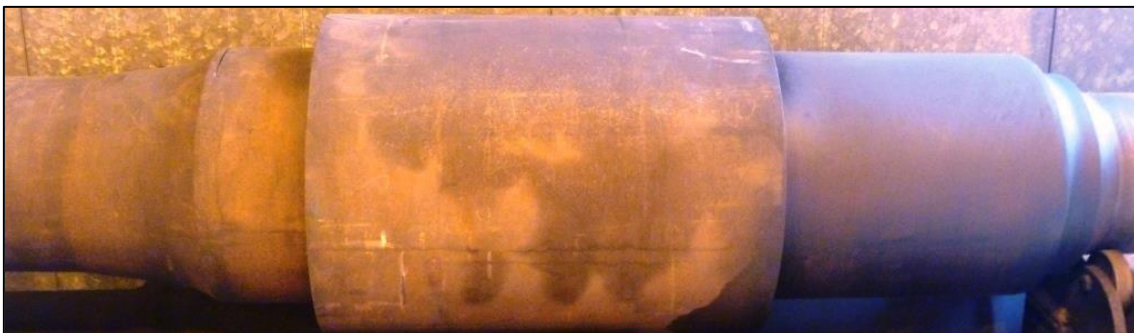
Figure 12: Tangara axle ultrasonic testing reference standard
